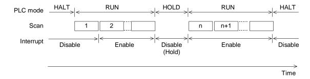
In the RUN mode, interrupt operation is disabled at the first scan, and enabled from the second scan.
